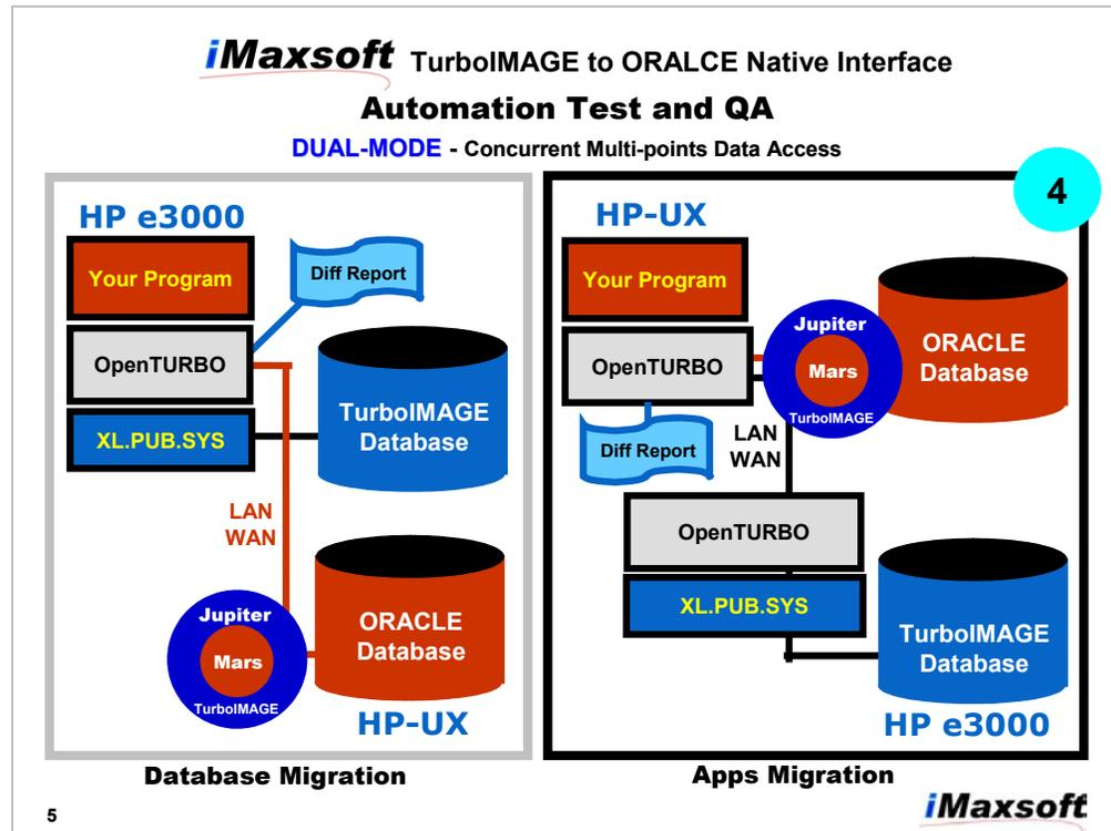
OPENTURBO Real-time Data Replicator translates TurboIMAGE calls into ORACLE SQL statements and applies updates to both ORACLE and TurboIMAGE simultaneously in 2PC (2 Phase Commit) mode or in off-line log-recovery mode.
