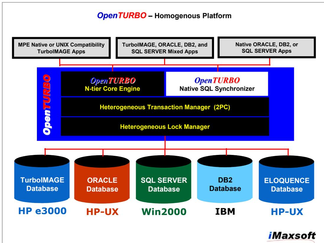
IMAXSOFT OPENTURBO provides a homogenous platform on heterogeneous environments. IMAXSOFT's migration platform is a mix of HP3000, HP-UX, LINUX, AIX, IMAGE, ORALCE, SQL SERVER, ELOQUENCE, and DB2; on our platform, you can direct your applications to run under any OS and to access one or more data sources concurrently at anytime; our goal is
