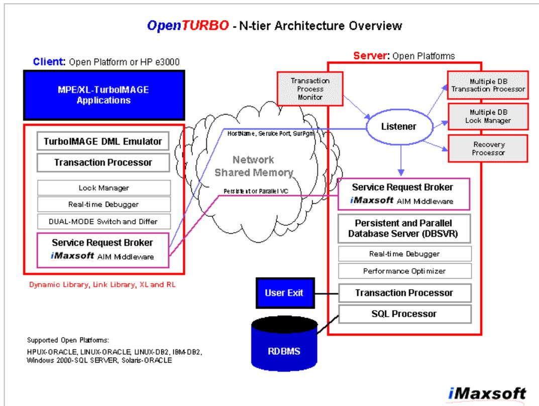
OPENTURBO is a n-tiers client-server architecture, it consists of TurboIMAGE emulator that is used by your existing HP3000 programs to access ORACLE on HP-UX as they were accessing TurboIMAGE on MPE/XL; a set of relational database transformation utilities that is used to replicate and move your entire TurboIMAGE database to ORACLE on HP-UX; and data integrity objects and toolsets that are used to support the co-existence of native relational database and OPENTURBO emulated applications.
