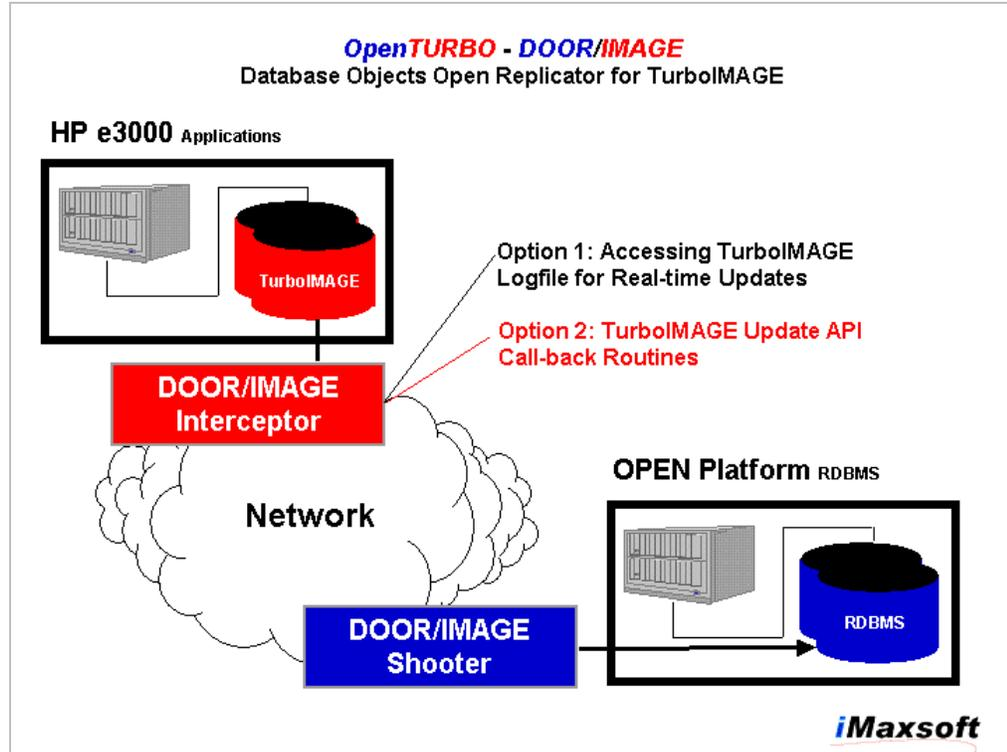
If you need to maintain both TurboIMAGE and ORACLE databases in-sync at all time, you want to maintain an exact mirror of TurboIMAGE in ORACLE on HP-UX, and you want 100% transparency to your applications, DOOR is solution; it is a database to database replication tool, it supports both real-time and office-line replication capabilities and it can replicate to multiple RDBMS on multiple server concurrently.
