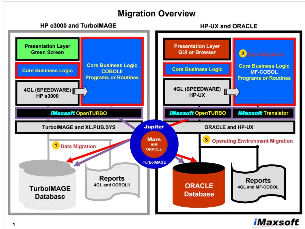
The above chart illustrates how data synching is done cross-platforms and cross-DBMS in real-time at application level. The application level data synching is required for bi-directional data synchronization in order to preventing infinite loop and racing problem.
