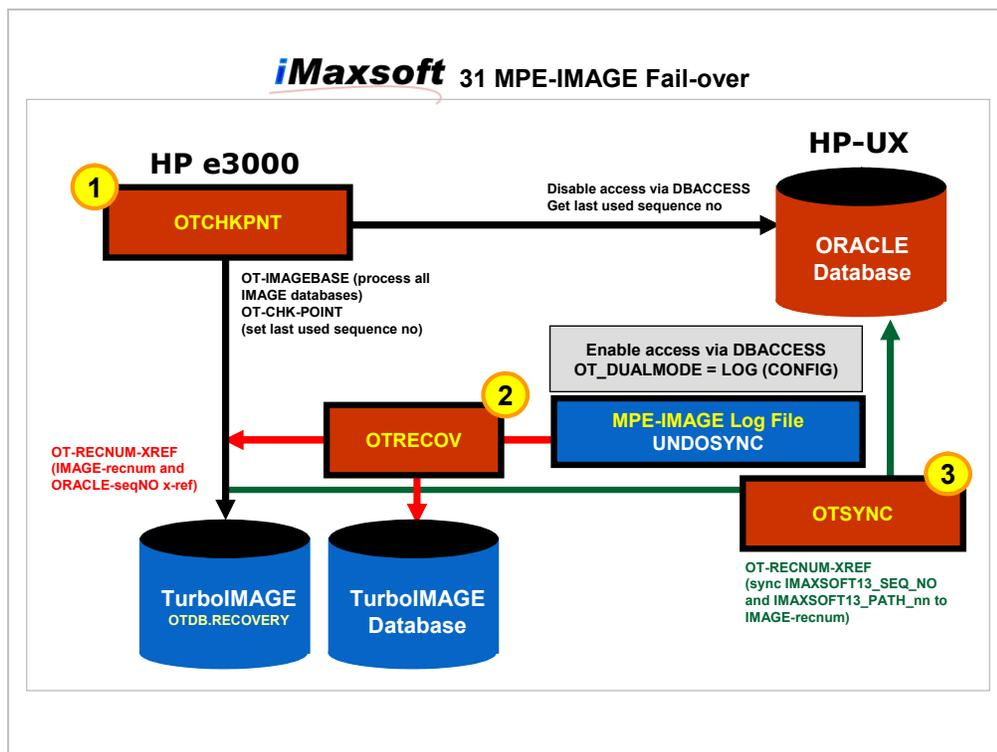
FAIL-OVER processor is mainly for off-line data replication and fall-back recovery, since it is off-line, the impact to the source servers are very minimum and major performance boost when transfer real-time sync to off-line sync.
